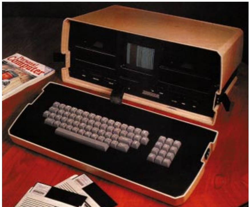
Oh, for those pioneering days of the Osborne 1: note the huge 3in screen!
